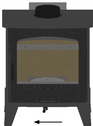
Air control fully closed
