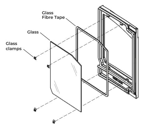
Ensure the door is on a soft flat surface before removing the glass. Unscrew the four glass clamps. Remove the old glass and glass fibre tape. Fit the new glass and glass fibre tap and glass clamps. The glass clamps should only be finger tight to allow for the expansion and contraction of the glass.
