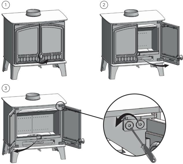
Loosen both screws as shown above in image 3. Ensure the door is supported at all times.
