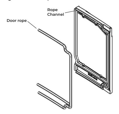
Ensure the door is on a soft flat surface before removing the door rope. Remove the door rope. Scrape away any old adhesive. Use a brush or dry cloth to remove any debris in the rope channel. Spread the rope glue evenly in the channel. Press the new rope into the rope channel and allow sufficient time to cure.
