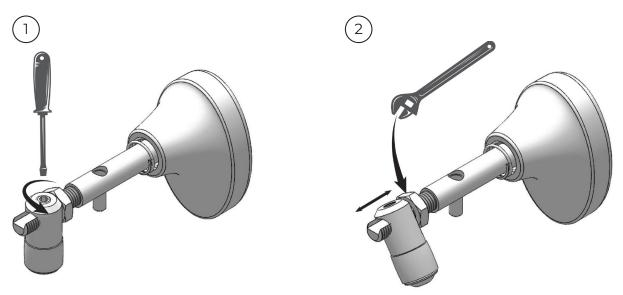
To adjust the handle remove the grub screw as shown in figure 1 above. Then loosen the nut shown in figure 2. This enables the door catch to be turned clockwise or anti-clockwise to move it forwards or backwards depending on the adjustment required. Once the desired setting is achieved re-tighten the nut and replace the grub screw.
