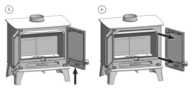
Once the top hinge is removed lift the door so that is clears the bottom hinge pin as shown in image 5. Then remove the door as shown in image 6. Repeat this process for the opposite door.
