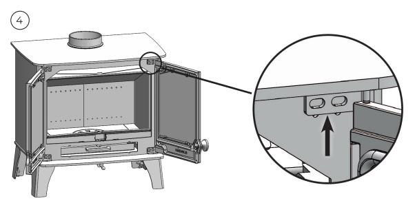
This will allow the hinge to be moved up and removed as shown in image 4 above.
