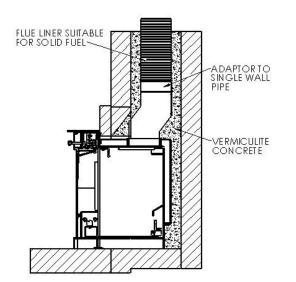
*If connecting to an existing masonry* chimney it is recommended that a flue forming pipe (short length of flue pipe) is used and the void between the flue forming pipe and the chimney is filled with vermiculite concrete.
