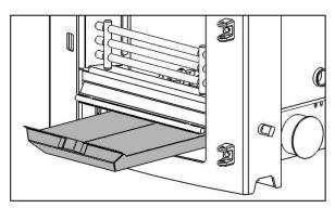
Remove the fuel retainer by lifting upwards of its supports and remove from firebox.
