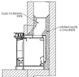
Alternatively a connection can be made using a register plate although it will be necessary to allow access for fitting the flue pipe to the register plate, infilling with vermiculite concrete and sealing all joints.
