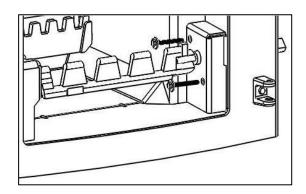
7. Remove the cam bar and cam bar cover by lifting the cam bar from the left hand side until clear of the support. Slide the cam bar to the left and remove.
