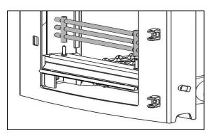
Remove the fuel retainer support (front plate) by lifting the fuel retainer support clear from its locating slots. Then remove.
