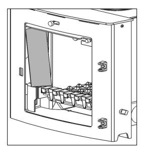
Remove the grate bars by lifting the front up off the cam bar and sliding forward off the rear grate support and lifting out of the firebox. Repeat with remaining grate bars.
