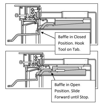
The baffle will automatically slide back into its closed position when the door is closed. This is achieved by the door pushing onto the baffle arm.
