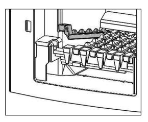
Remove cam bar by removing the two M6 x 50mm screws form the cam bar cover.
