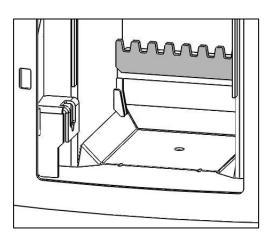
9. Remove the baffle by sliding it forward until it reaches its stop. Then lift and slide forward until clear of its supports and lower into the firebox.
