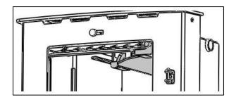
To slide the baffle forward you will need to use the tool provided. Hook the tool onto the tab at the front of the baffle and pull forward until it hits the stop. This will create a 30mm gap at the back of firebox.
