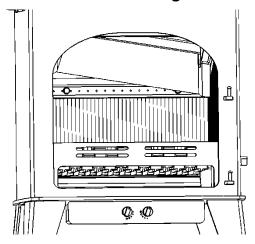
To install the Baffle, slide the left-hand end of the Baffle up, and over the support. Push the Baffle to the left until the right-hand edge clears the other support. Slide the Baffle back to the right until it sits centrally in the stove. Check that the two tabs at the front of the Baffle are between the Baffle Supports.
