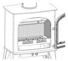
1. Remove Front Plate by lifting it up out of the slots on either side. Rotate to remove from the stove.
