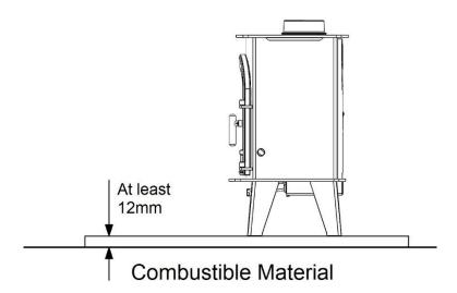
The hearth should extend at least 150 mm from the sides and rear of the stove, and at least 225 mm from the front of the stove.
