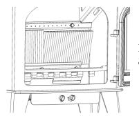
Pull the top edge of each Rear Brick forward and lift the brick out of the Stove.
