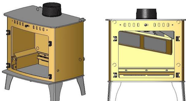
Remove the Ashpan, Riddling Bars, Cam Bar and Catch Bar. Lift the Baffle Brick and slide to the left. When the right side of the Brick clears the Baffle Support, lower the Brick into the Fire Box and remove.
