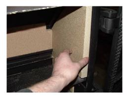
Remove all of the Riddling bars. Slide the front of the Side Brick towards the centre of the Stove and remove the Side Brick.
