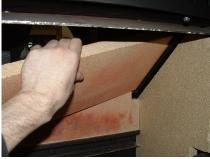
Lift the Baffle Brick and slide to the right. When the left side of the Brick clears the Baffle Support, lower the Brick into the Fire Box and remove.
