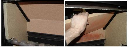
Lift the Baffle Brick and slide to the right. When the left side of the Brick clears the Baffle Support, lower the Brick into the Fire Box and remove.
