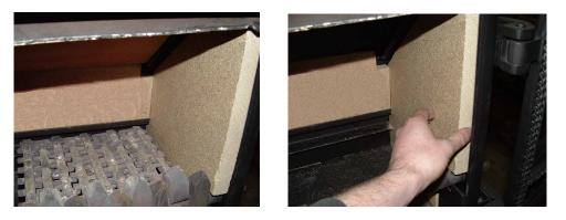
Remove all of the Riddling bars. Slide the front of the Side Brick towards the centre of the Stove and remove the Side Brick.
