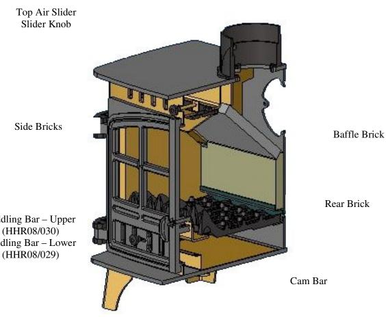
Flue Collar (HHR08/023) Flue Cover (HHR08/024)
