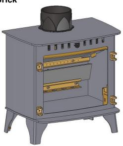
Pull the top edge of the Rear Brick towards you, lift and remove.
