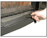
To burn wood, push the operating tool up and away from you. When left in this position, air is directed through the slots now formed behind the door, and not through the firebed, which now provides a solid base to build up a bed of ash. Surplus ash can be removed either by gentle riddling or with a shovel.
