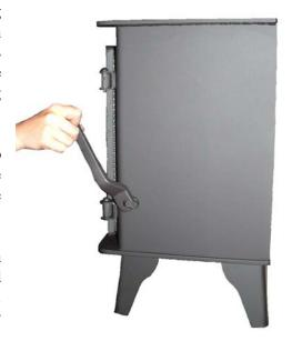
**To burn wood**, push the operating tool up and away from you. When left in this position, air is restricted through the bed of the fire providing a solid base to build up a bed of ash. Surplus ash can be removed either by gentle riddling or with a shovel.
