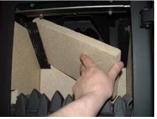
Lift the Baffle Brick and slide to the left. When the right side of the Brick clears the Baffle Support, lower the Brick into the Fire Box and remove.
