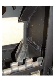
Remove all of the Riddling bars. Slide the front of the Side Plate Fabrication towards the centre of the Stove and remove the Side Brick. Also remove the Side Plate.
