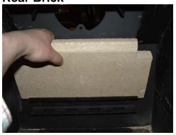
Pull the top edge of the Rear Brick towards you, lift and remove.
