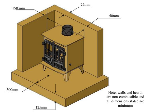
Note that combustible material refers to any material that will degrade when exposed to high temperatures.
