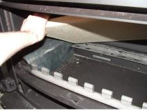
Remove the four furthest grate bars on the left-hand side.
