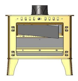
Lift the Baffle Brick and slide to the left. When the right side of the Brick clears the Baffle Support, lower the Brick into the Fire Box and remove.
