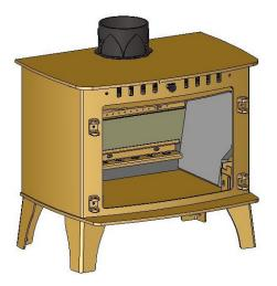
Remove all the Riddling Bars, Ashpan, Cam Bar and Catch Bar.
