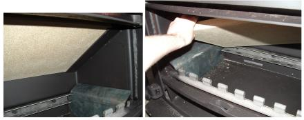
Remove the four furthest grate bars on the left-hand side. Lift the Baffle Brick and slide to the right.
