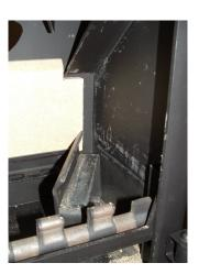
Remove all of the Riddling bars. Slide the front of the Side Plate Fabrication towards the centre of the Stove and remove the Side Brick. Also remove the Side Plate.
