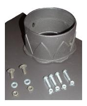
Place the Flue Gasket on the top, or rear outlet as required. Place the Flue Collar on top of the Gasket. Secure to the four locating tabs, inside the flue outlet, using the M6 nuts & bolts supplied. Fit the 2 - M8 carriage bolts, washers & nuts into the Damper Holes, located on each side of the Flue Collar.
