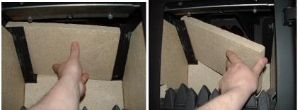
Lift the Baffle Brick and slide to the left. When the right side of the Brick clears the Baffle Support, lower the Brick into the Fire Box and remove.
