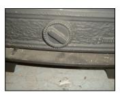
It is important that the riddling tool is used to remove the ash to ensure airflow through the firebed and allow the fire to burn over the entire area of the grate.
