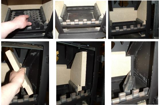
Remove all of the Riddling bars. Slide the front of the Side Plate Fabrication towards the centre of the Stove and remove the Side Brick. Also remove the Side Plate.
