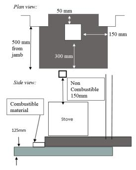
The stove can be recessed in a suitable sized fireplace but a permanent free air gap of at least 150mm on top and 50mm at the sides (although we recommend 150mm for the sides and 50mm at the back of the stove to obtain maximum heat output and for access to the rear of the stove.)
