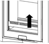
3. Remove the baffle brick by lifting it up, sliding it to the right and then lowering the left-hand edge into the firebox
