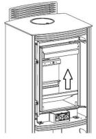
7. Remove the Air Valve Cassette by removing the socket screws holding it in place, turning both air controls to the fully open position (clockwise) and then gently pulling on the fascia to slide the cassette out from under the firebox.
