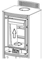
5. Remove the three rear brick (Eco R3) and the two rear brick (Eco R5) sections noting their positions and orientation.
