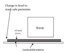
If the stove is not to stand in a recess, it may stand wholly above a hearth made of noncombustible board / sheet material or tiles, at least 10mm thick.
