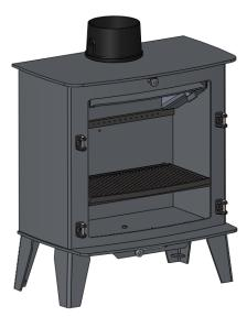
10) Remove the baffle by lifting the left hand side and sliding it to the left until the right hand side is clear of the support.
