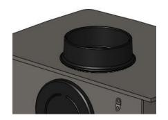
Wind the eight M6 studs supplied into the fixing holes in the flue collar and blanking plate until finger tight. Place the gasket in position on the top plate of the stove and lower the flue collar or blanking plate (as required) on to the stove top, taking care to line up the studs with the fixing holes. Secure in place using the M6 nuts and washers.
