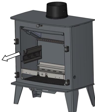
7) Remove the front plate (on double door stoves, the front plate should be pushed back slightly to disengage it from the locating fork).
