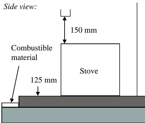
The stove can be recessed in a suitable sized fireplace but a permanent free air gap of at least 150mm on top and 50mm (although we recommend 150mm) around the sides and 50mm at the back of the stove to obtain maximum heat output and for access to the rear of the stove. The hearth should extend at least 300 mm from the front of the stove. The stove should stand wholly above a solid, non-combustible hearth, at least 125 mm thick (this may include the thickness of a solid floor).
