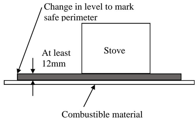
If the stove is not to stand in a recess, it may stand wholly above a hearth made of non-combustible board / sheet material or tiles, at least 12mm thick.
