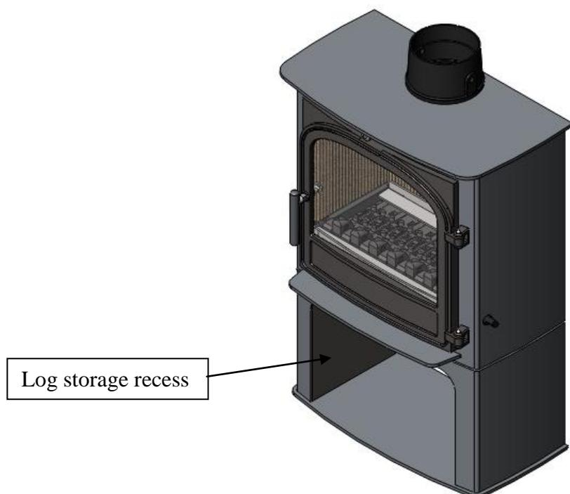
Fuel may be placed in the log storage recess underneath the European variant. The logs should be stacked in such a way that they do not touch the heat shield at the top of the recess.
