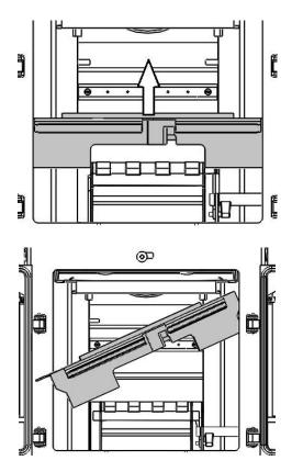
11. Detach the cam bar linkage arm from the front cam bar, rotate the cam bar and lift it out.
