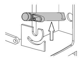
12. Lift out the rear cam bar along with the cam bar linkage arm.
