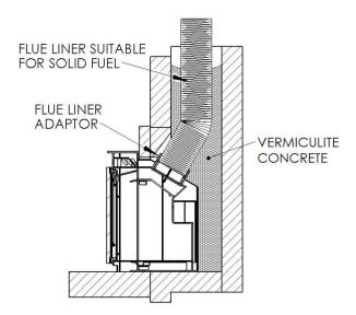
If connecting to an existing masonry chimney it is recommended that a flue forming pipe (short length of flue pipe) is used and the void between the flue forming pipe and the chimney is filled with vermiculite concrete.
