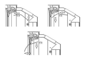
8. Remove the grate bars, starting with the high bars.
