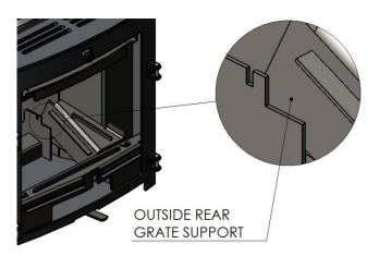
Lower the side plate into position so that the top surface of it is flush with that of the front plate/catch bar as shown.
