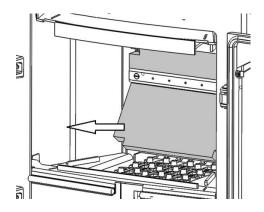
6. Remove the lower rear brick support using the finger hole provided to lift it from its slots.
