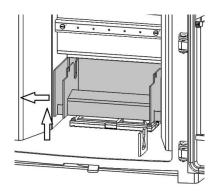
14. Lift out the primary air valve slider.
