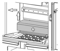
7. Cut the cable ties and remove the baffle by rolling it up over the baffle supports and out of the stove.
