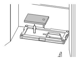
15. Undo the four M6 x 25mm screws and remove the primary air valve and gasket.
