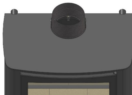
Wind the four M6 studs supplied into the fixing holes in the flue collar until finger tight. Place the flue collar onto the stove and tighten using the supplied washers and nuts from inside the stove.
