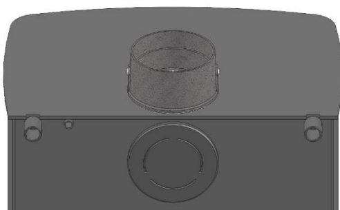
Place the gasket on the outlet and put the blanking plate on top of this. Wind the four M6 studs supplied into the fixing holes until finger tight. Place the plate onto the stove and tighten using the supplied washers and nuts from inside the stove.
