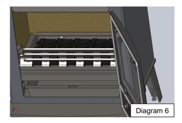
The Baffle can now be replaced.
