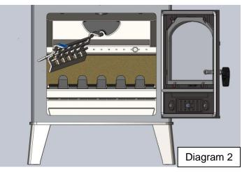
Fit the Multi-Fuel Extension as shown in Diagrams 2, 3, and 4.
