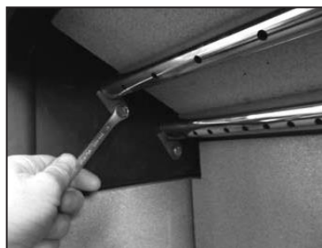
8mm bolt holding cam latch
