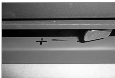
Air lever shown in the closed position
