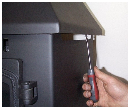
Figure 10: Tightening The Canopy
