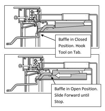
The baffle will automatically slide back into its closed position when the door is closed. This is achieved by the door pushing onto the fixing on the baffle arm.
