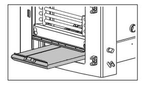
2. Remove the fuel retainer by lifting off of its supports and remove from firebox.
