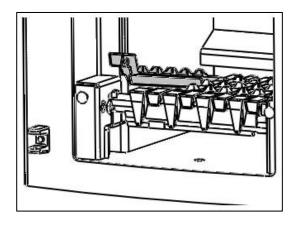
6. Remove the baffle by sliding it forward until it reaches its stop. Then lift and slide forward until clear of its supports and lower into the firebox.
