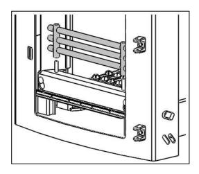
Remove the catch bar (front plate) by lifting until the widest section of the keyhole slots are in line with the catch bar supports. Then pull forward until clear of the supports and remove.
