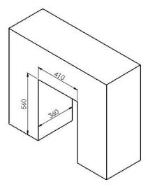
This appliance will fit into a standard 16" fireplace opening if the clay fire back is removed.
