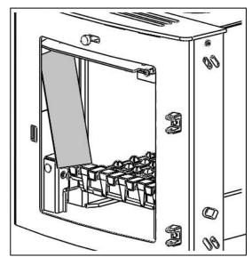
5. Remove the grate bars by lifting the front up off the cam bar and sliding forward off the rear grate support and lifting out of the firebox. Repeat with remaining grate bars.
