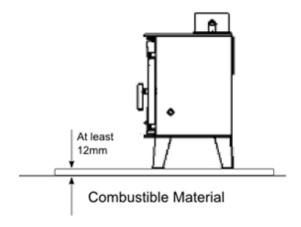
The hearth should extend at least 150 mm from the sides and rear of the stove, and at least 300 mm from the front of the stove.
