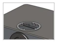
Place a flue gasket in position on the top plate of the stove and lower the flue collar or blanking plate (as required) on to the stove top, taking care to line up the studs with the fixing holes.
