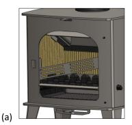
3. Remove the baffle by pulling it forwards and sliding it to the left until the right side of it clears the baffle support and then lowering it into the firebox and removing it (b).
