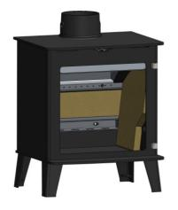
Slide the base of the Side Brick towards the centre of the stove and remove.
