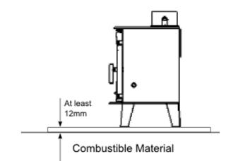
The hearth should extend at least 150 mm from the sides and rear of the stove, and at least 225 mm from the front of the stove.
