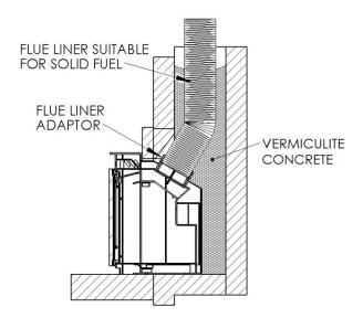
If connecting to an existing masonry chimney it is recommended that a flue forming pipe (short length of flue pipe) is used and the void between the flue forming pipe and the chimney is filled with vermiculite concrete.
