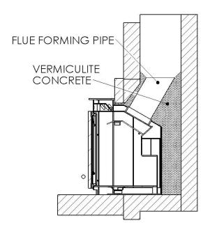
Alternatively a connection can be made using a register plate although it will be necessary to allow access for fitting the flue pipe to the register plate, infilling with vermiculite concrete and sealing all joints.
