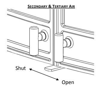
Secondary air is controlled via the slider above the door(s) (slide right to open), it is this "Airwash" that keeps a clean and uninterrupted view of the fire.
