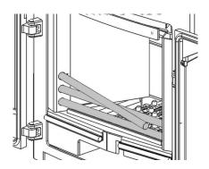
3. Remove the fuel retainer supports by lifting them free from the slots in the catch bar and swinging the bottom ends out of the stove.
