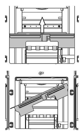
11. Detach the cam bar linkage arm from the front cam bar, rotate the cam bar and lift it out.
