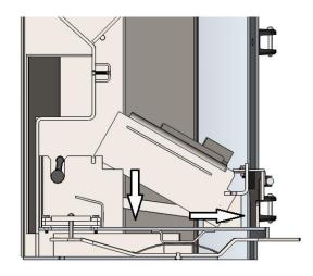
Ensure that the back end of the side plate is outside the rear grate support as shown.
