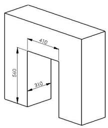
This appliance will fit into a standard 16" fireplace opening if the clay fireback is removed.
