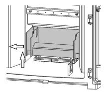
14. Lift out the primary air valve slider.
