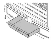
Remove the fuel retainers by turning them towards you until the pins at the ends of them align with the cut-outs in the fuel retainer supports and sliding them out.
