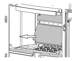
6. Remove the lower rear brick support using the finger hole provided to lift it from its slots.
