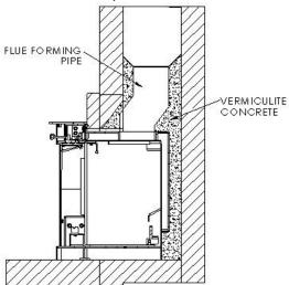
Alternatively a connection can be made using a register plate although it will be necessary to allow access for fitting the flue pipe to the register plate, infilling with vermiculite concrete and sealing all joints.
