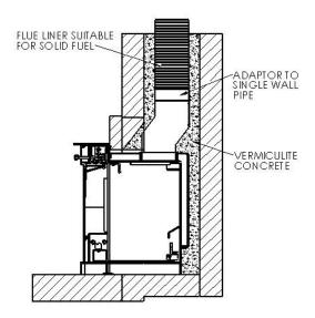
If connecting to an existing masonry chimney it is recommended that a flue forming pipe (short length of flue pipe) is used and the void between the flue forming pipe and the chimney is filled with vermiculite concrete.
