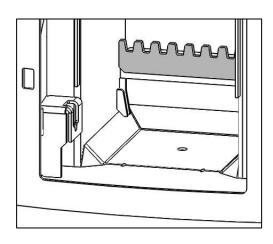
Remove the baffle by sliding it forward until it reaches its stop. Then lift and slide forward until clear of its supports and lower into the firebox.
