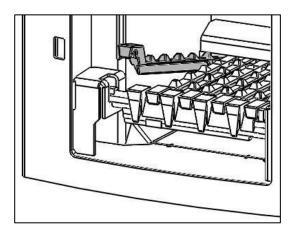
6. Remove cam bar by removing the two M6 x 50mm screws form the cam bar cover.
