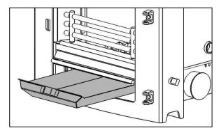
Remove the fuel retainer by lifting upwards of its supports and remove from firebox.
