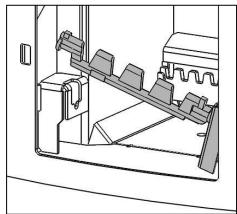
Remove the rear grate bar support by lifting the grate bar support clear of the locating slots and remove.
