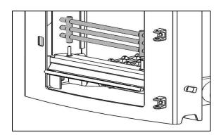
3. Remove the fuel retainer support (front plate) by lifting the fuel retainer support clear from its locating slots. Then remove.
