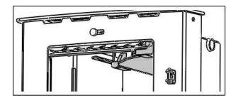
To slide the baffle forward you will need to use the tool provided. Hook the tool onto the tab at the front of the baffle and pull forward until it hits the stop. This will create a 30mm gap at the back of firebox.
