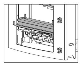
4. Remove the bricks by sliding forward so they are clear of their supports and tilting the bottom edge into the fire box.
