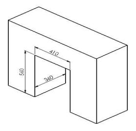
This appliance will fit into a standard 16" fireplace opening if the clay fire back is removed.
