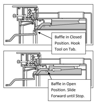
The baffle will automatically slide back into its closed position when the door is closed. This is achieved by the door pushing onto the baffle arm.
