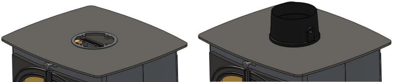
Place the Flue Gasket on the Top Plate Flue Exit. Place the Flue Collar on top of the Gasket. Secure to the four locating tabs, inside the flue outlet, using the M6 nuts & bolts supplied. Fit the 2 - M8 carriage bolts, washers & nuts into the Damper Holes, located on each side of the Flue Collar.
