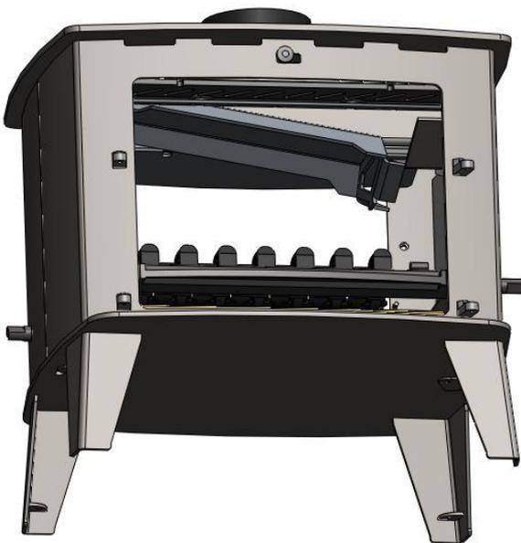
Remove the Location Pins from Turbo Bar. Slide it to the left. Once clear of the R.H. Turbo Duct pull it towards you and out of the L.H. Turbo Duct.
