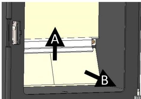
5. Remove the bottom rear brick by pushing the brick upwards (A). Then pull the bottom edge of the rear brick forward and lift the brick out of the stove.
