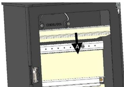
4. Remove the brick/steel baffle by dropping down into the firebox (A) and then remove the other side brick.
