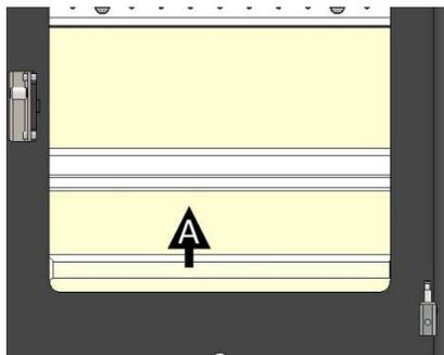
2. Remove the bottom base brick by lifting up the front (A), twist and slide out of body of stove.
