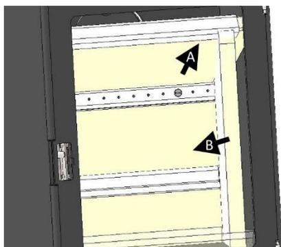
3. Lift up the baffle on one side (A) remove one side bricks, taking care not to disturb the top rear bricks. Pull front forward (B) and then remove the brick from the stove.
