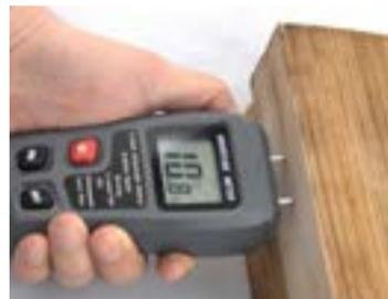
Used to measure moisture content of fuel.
